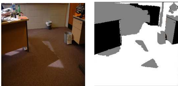
Figure 7. The left image is an indoor scene and the image on the right shows the illuminant map recovered: outdoor (gray), indoor (black) and mixed (white).
